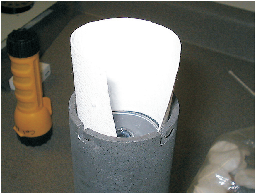
Figure 22 Place fiber ceramic paper to center the cell in cell basket.
