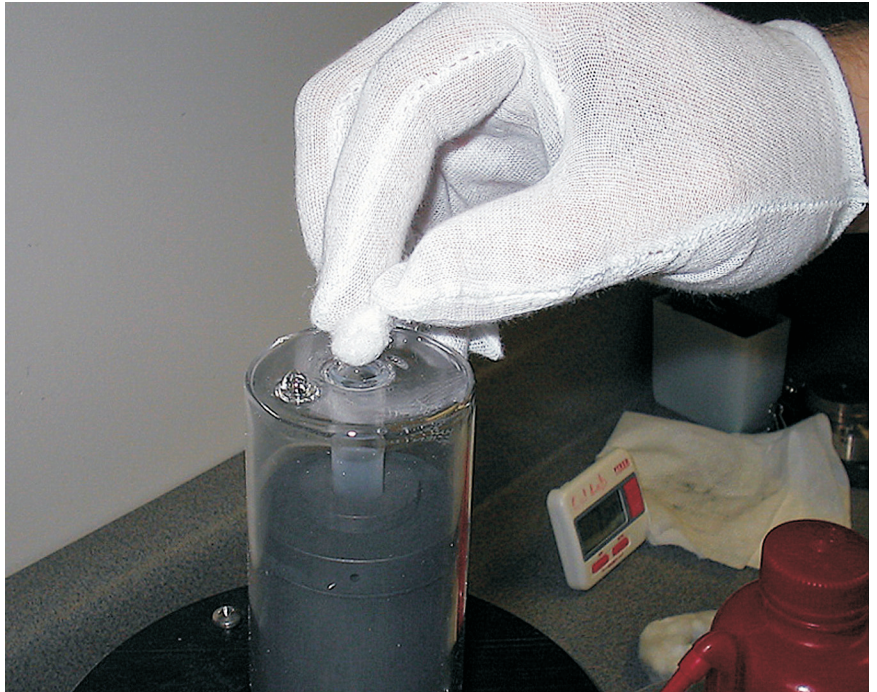
Figure 14 Place insulation in re-entrant well.
