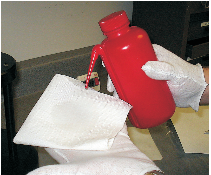
Figure 12 Preparing paper towel with reagent grade alcohol.
