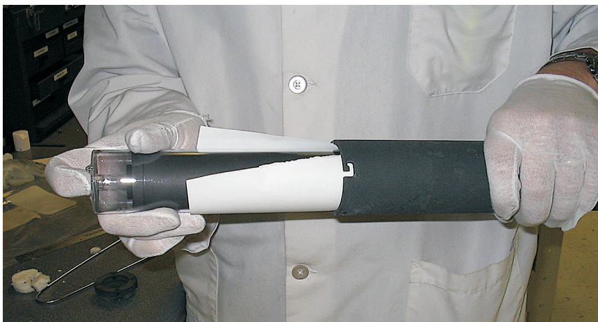
Figure 21 Insert cell into basket.
