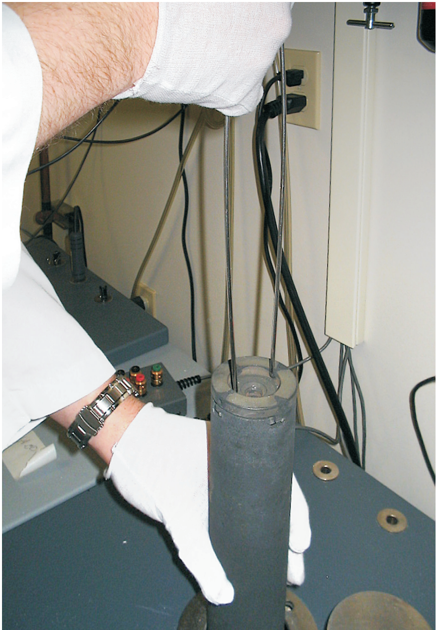
Figure 26 Installing basket assembly in furnace.
