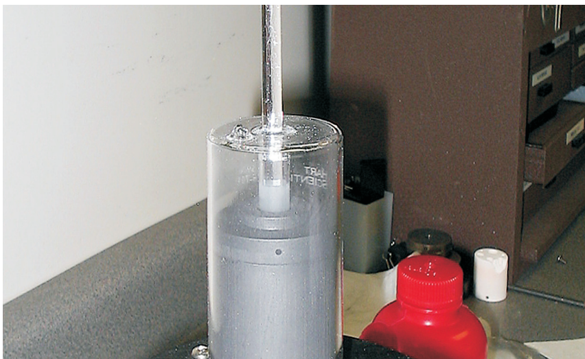
Figure 15 Push insulation to bottom of re-entrant well.
