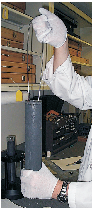
Figure 25 Preparing basket assembly for installation in furnace.
