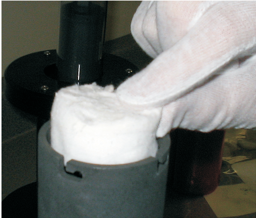
Figure 17 Place insulation in cell basket
